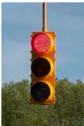
LED Traffic Signal
